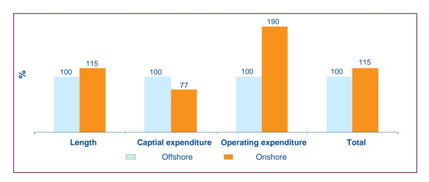
Total costs of an offshore pipeline are **some 15% lower** than an onshore pipeline, calculated over an period of 25 years
